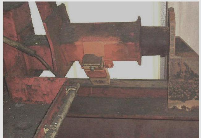
Haftblock an Kranschiene
